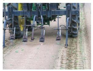
Figure 6. Broadcast flame weeder
