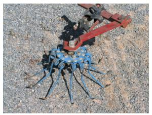
Figure 8. Flexible spider weeder
