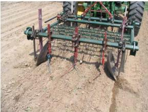
Figure 5. Flex-tine weeder with torsion rods
