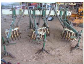
Figure 10. Rolling unit-two-row unit
