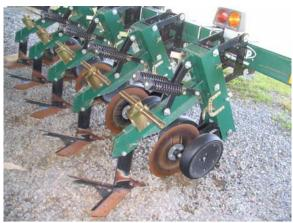
Figure 3. High residue cultivator
