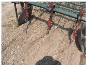
Figure 9. Torsion weeder—two pairs of torsion rods adjusted for twin row cabbage
