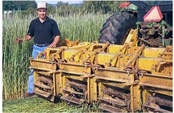
Open blade Buffalo stalk chopper modified by Steve Groff, Cedar Meadow Farm, Lancaster County, PA.
