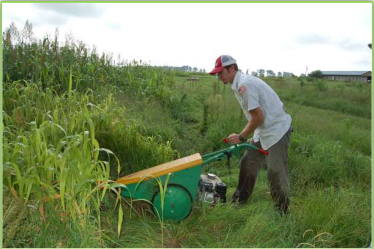
“Walk behind“ equipment can be used to harvest and remove nutrients deposited into the system.
