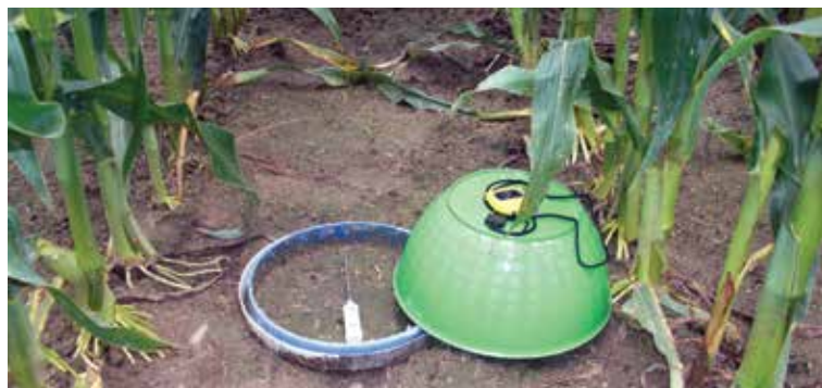
After rainfall events, gas collection units like these are used to measure greenhouse gas emissions in the FSRU. Photo: Tomas Moreno/CEFS
