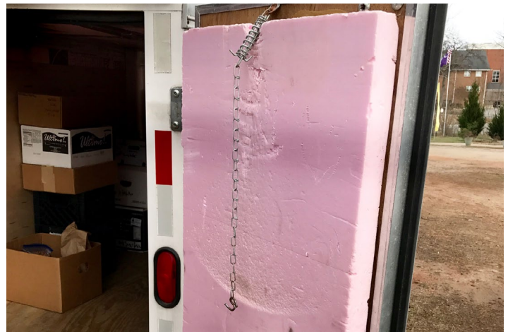
Photo 3.7. Interior of the mobile cooler with plywood floor and walls, XPS insulation, an A/C unit and taped sides.
